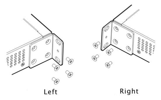
Align the mounting holes in the mounting bracket with the mounting holes in the rack, as shown in Figure 3-2.
