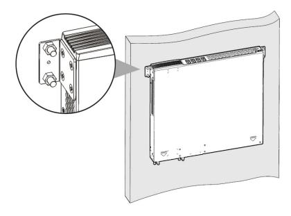
SUITABLE FOR MOUNTING ON CONCRETE OR OTHER NON-COMBUSTIBLE SURFACE ONLY.
