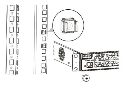
Use the supplied M6 screws and cage nuts to securely attach the mounting brackets to the rack, as shown in Figure 3-3.
